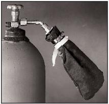
valve tightly and tap the cone gently to remove any ice sticking to it. The ice may be squeezed into a hard pack or left in flake form depending upon its intended use.
